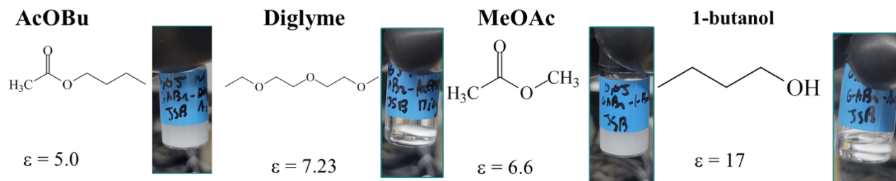
Figure S1. Solubility test of GABr. Each solvent structure is represented with their dielectric constant. On the right side, for each solvent, is shown the result of the dissolution process after one hour of stirring.
