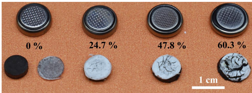
Figure S7. Photographs of CR927 coin cells subjected to constant-speed impact of 1 mm/min with 0^\circ placement at different strains.
