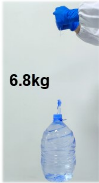
Fig. S11 Image of a single UBSY lifting 6.8 kg water.
