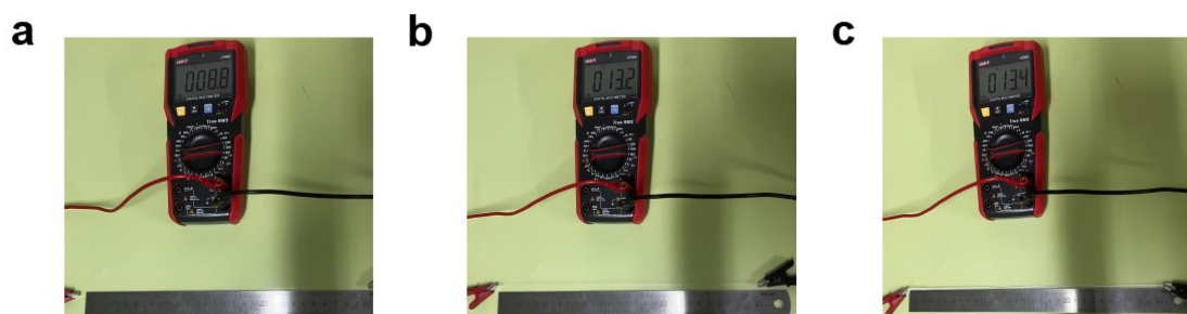
Fig. S6 Resistance measurement of 300 mm. a) Cu wire. b) UCY. C) UCPMY. d) Surface resistance of the UCPMY.
