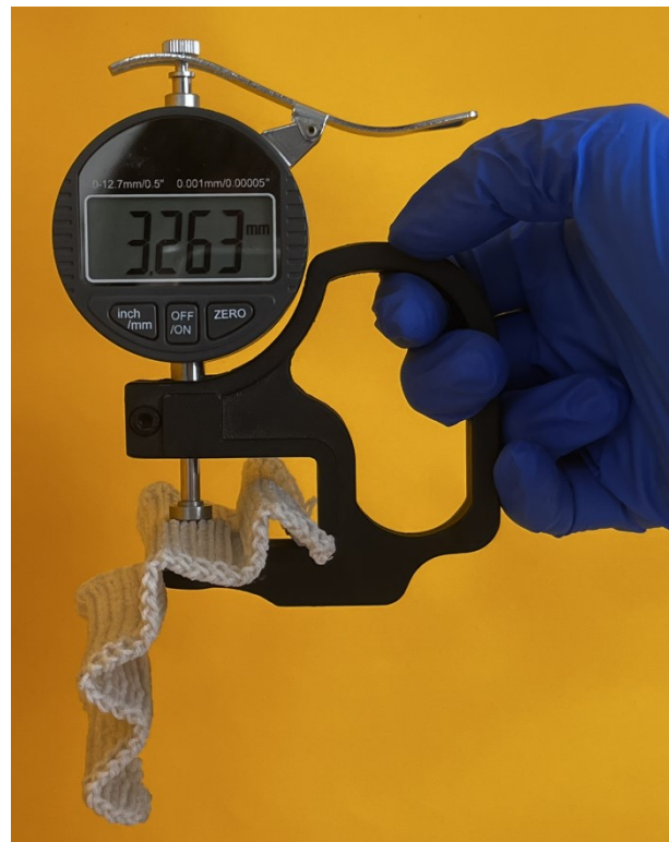
Fig. S12 Image of thickness test of the OSKF
