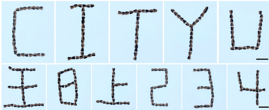
Fig. S5 Assembly of Micromotors into Sophisticated Patterns. English letters, Chinese characters, and numbers with encoded information are assembled with the assistance of a magnetic field. Scale bar, 2 mm.
