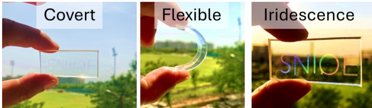
Fig. S12. The flexible photonic structure fabricated by replicating printed monolayer photonic structure (shown in inset Fig. 6c of the main manuscript) on PDMS using soft lithography.
