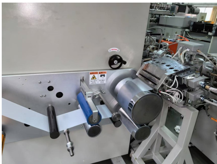
Fig. S3. Continuous production of DBPS using a dual-layer co-extrusion device
