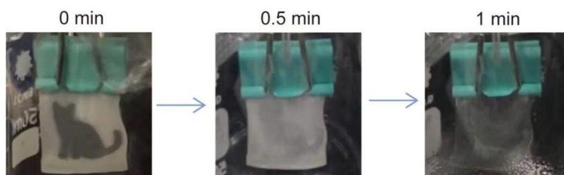
Fig.S10 Digital photograph of cat-shaped patterned film, encrypted in DCM vapor. The sorption of DCM can accelerate the information encryption process to 1 min, which is much more rapid than the drying-induced information encryption.
