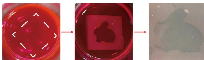
Fig.S8 Dye-staining experiments. The patterned film was immersed in acetone containing Rhodamine B. The pattern appears after 30 min of sorption of acetone. Upon drying, the non-crosslinking area is stained to become red, while the crosslinking area was not stained by dye.
