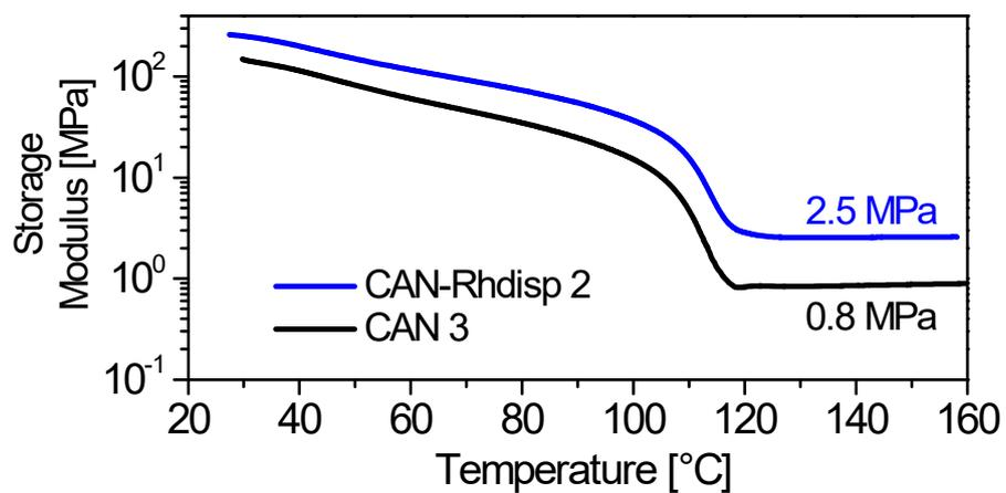
**Figure S9.** Storage Modulus vs Temperature of CAN-Rhdisp 2 and CAN 3. Tests are carried out on bars with nominal dimensions 6x1x30 mm<sup>3</sup>, cut from plates obtained by compression moulding
