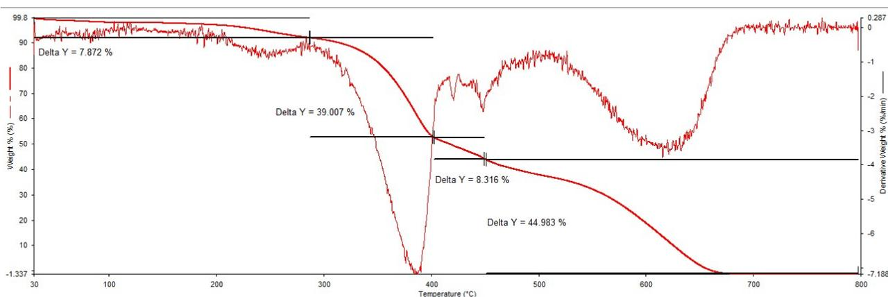
Figure S11. TGA measurement on Rhodamine 2
