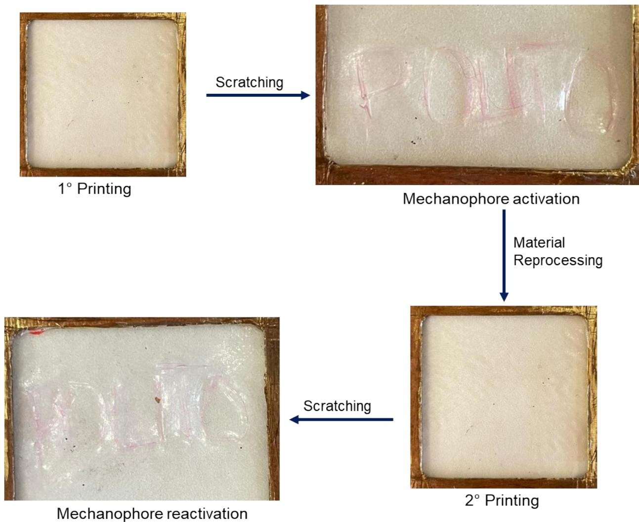
**Figure S18.** CAN-Rh 1 printing, activation, reprinting and reactivation test.
