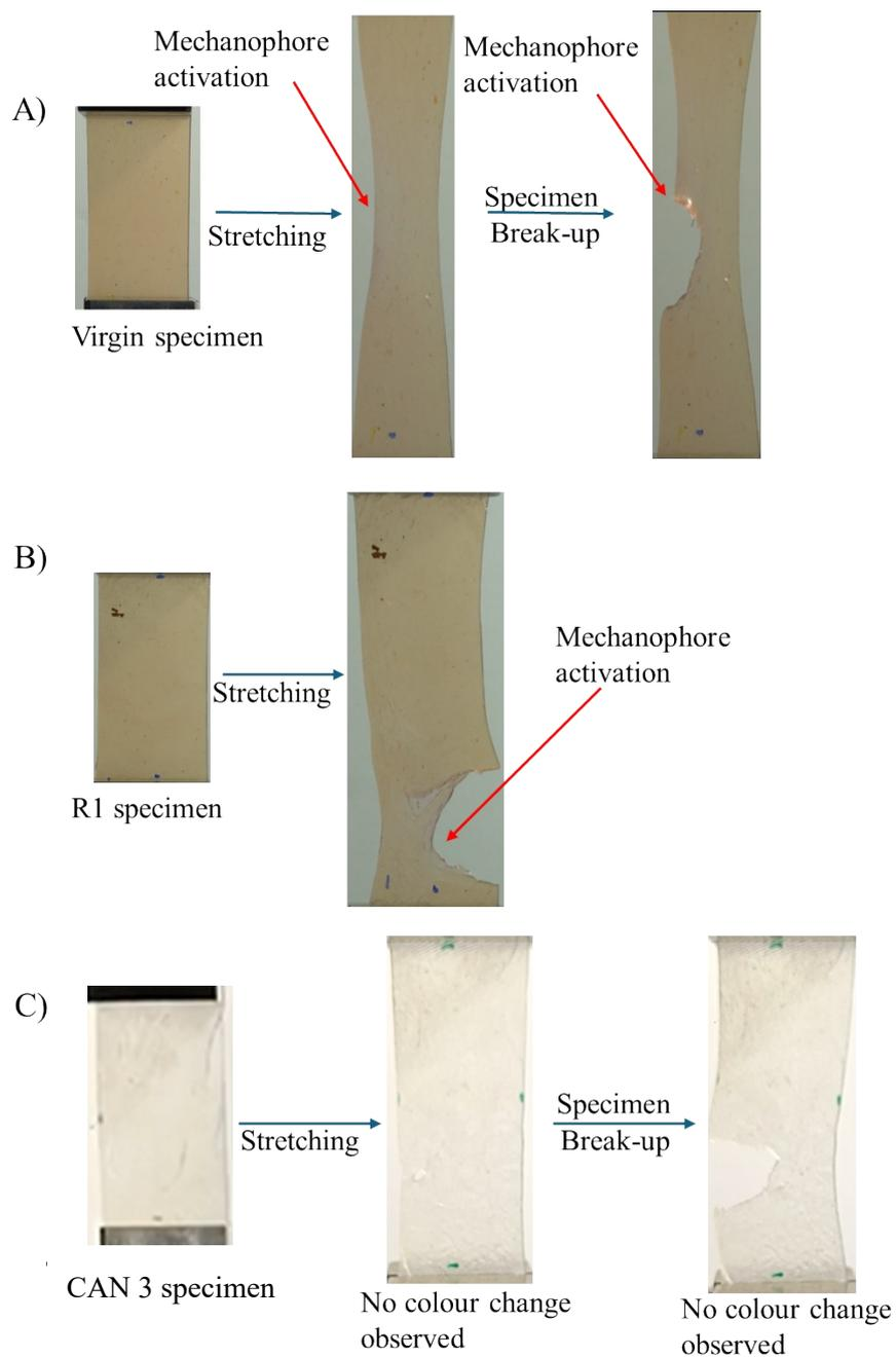
**Figure S16.** Self-reporting properties of A) virgin CAN-Rh 1 (V), B) recycled CAN-Rh 1 during stress-strain measurement; C) Control experiment with CAN-3 as reference.
