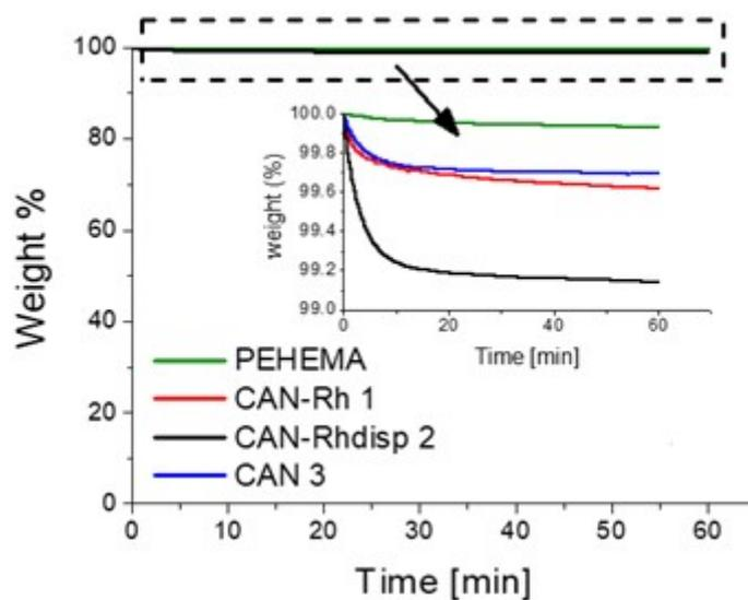
**Figure S14.** Isothermal (150°C) TGA measurement on CAN-Rh 1, CAN-Rhdisp 2 and CAN 3, compared to pristine PEHEMA. Inset shows large magnification to show minor weight loss difference between the different formulations
