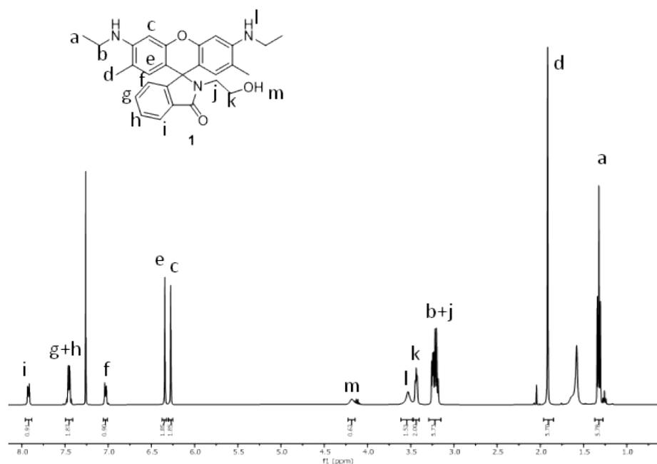
Figure S1. <sup>1</sup>H-NMR (CDCl<sub>3</sub>, 25°C, 400MHz) spectrum of Rhodamine 1
