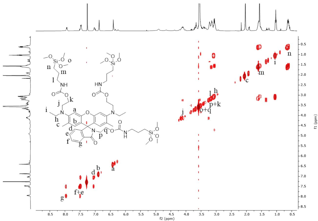
**Figure S4.** COSY-NMR ( $\text{CDCl}_3$ , 25°C, 400MHz) Spectrum of Rhodamine 3
