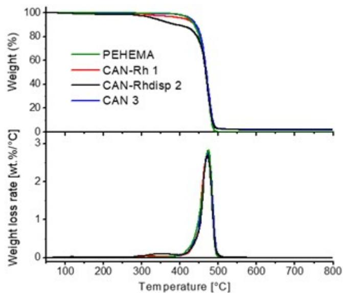
**Figure S13.** TGA measurement on heating (10°C/min) for CAN-Rh 1, CAN-Rhdisp 2 and CAN 3, compared to pristine PEHEMA
