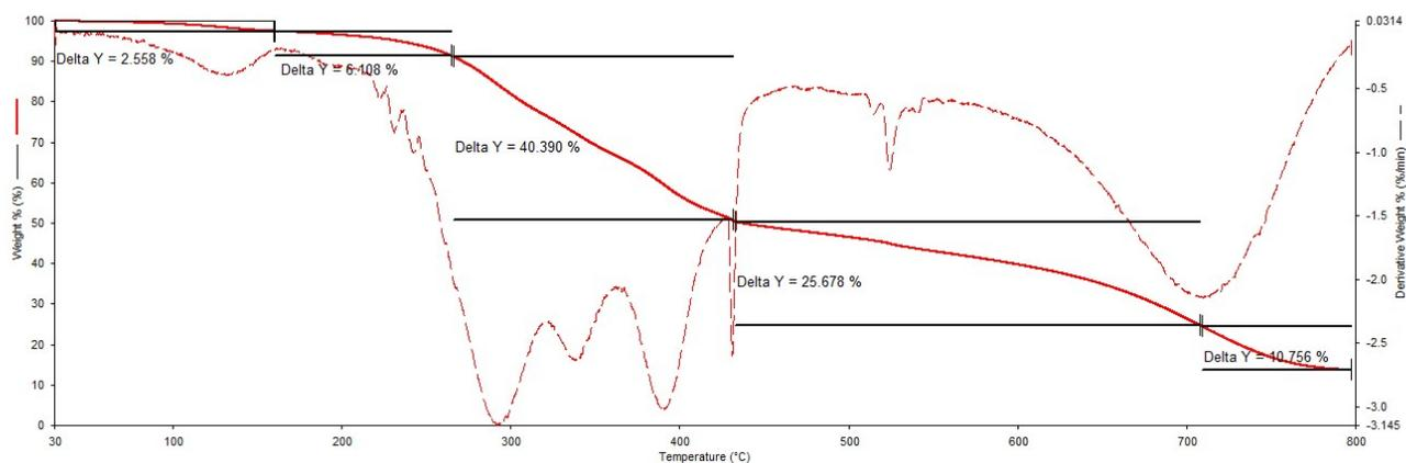
Figure S12. TGA measurement on Rhodamine 3
