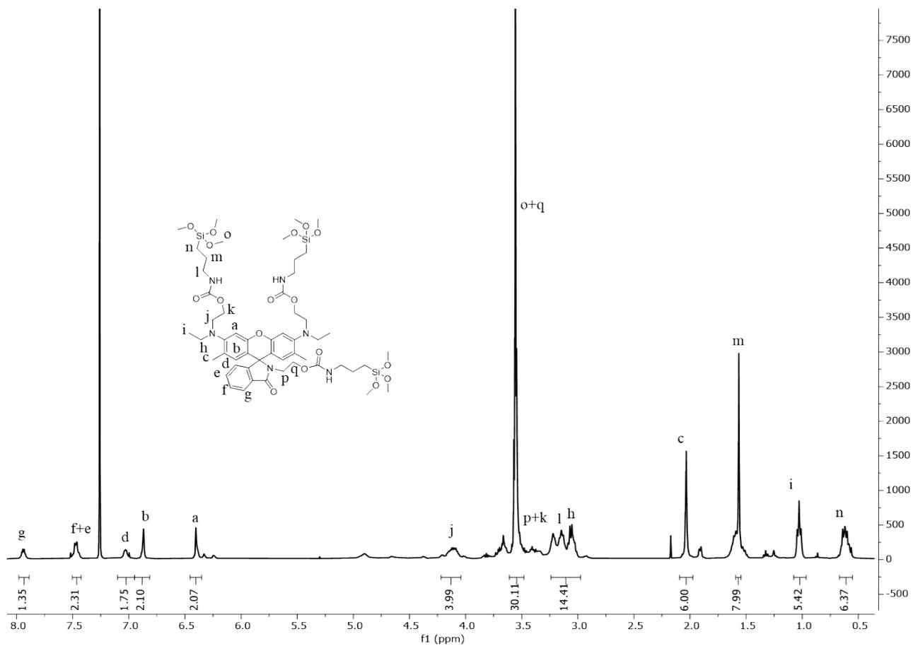
**Figure S3.** <sup>1</sup>H-NMR (CDCl<sub>3</sub>, 25°C, 400MHz) spectrum of Rhodamine 3
