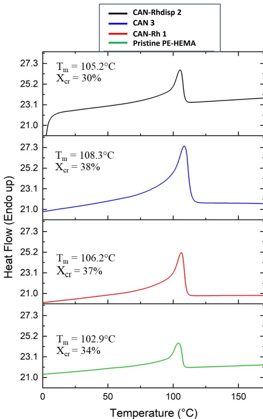
**Figure S8.** DSC second heating ramp of pristine PE-HEMA (green trace), CAN-Rh 1 (red trace), CAN 3 (blue trace), CAN-Rhdisp 2 (black trace).
