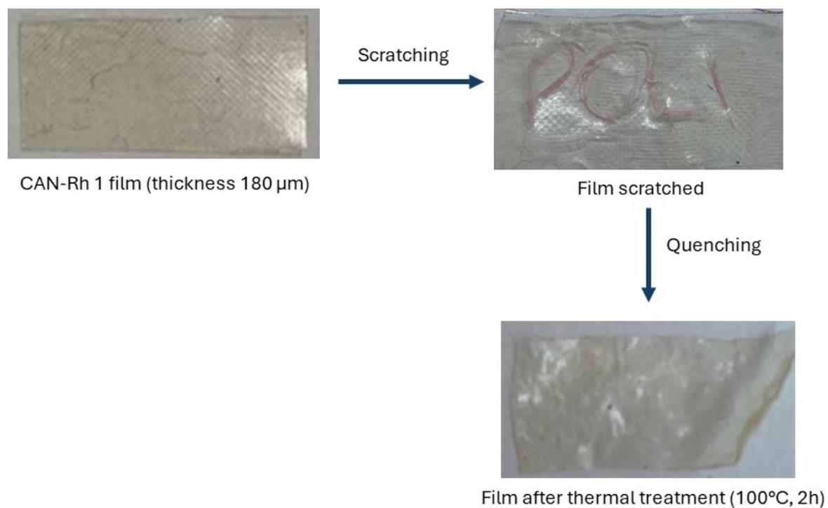
**Figure S17.** CAN-Rh 1 scratching and quenching test
