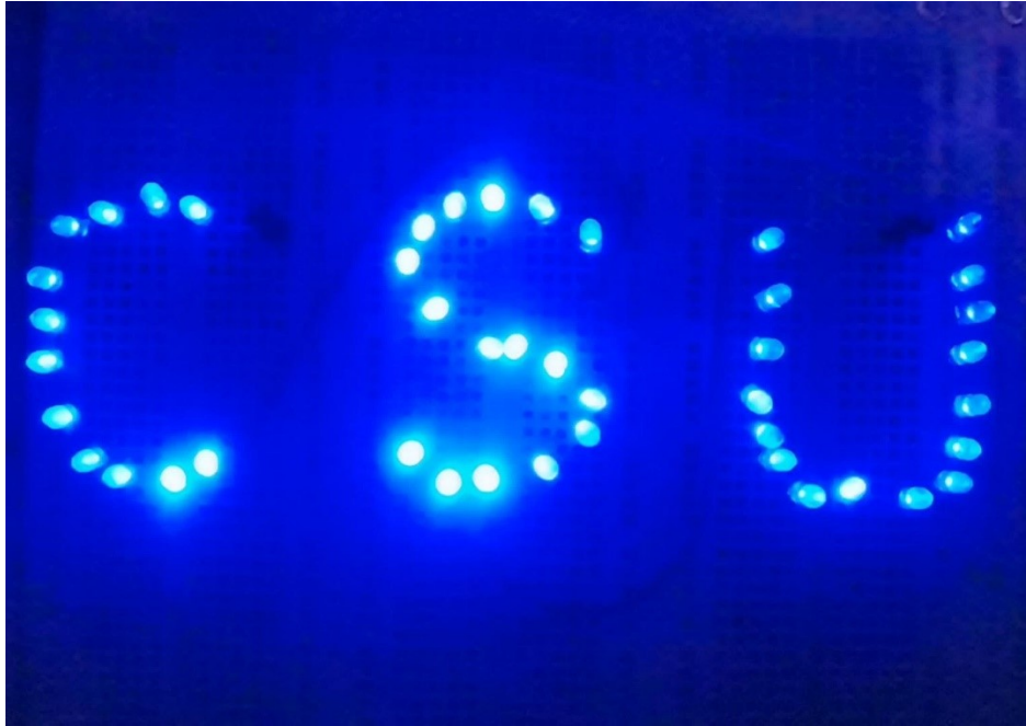
Fig. S7. Optical image showing 45 LEDs illuminated by piezoelectric energy harvester.
