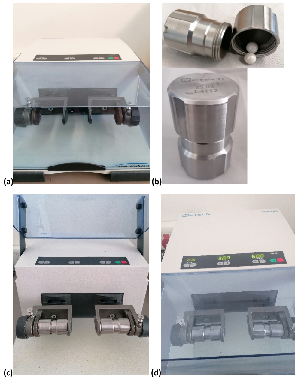
Fig. S26 (a) Retsch MM400 mixer mill without vessels; (b) open and closed 25 mL vessel; (c) Retsch MM400 mixer mill with vessels; (d) Retsch MM400 mixer mill with vessels and input synthesis parameters.
