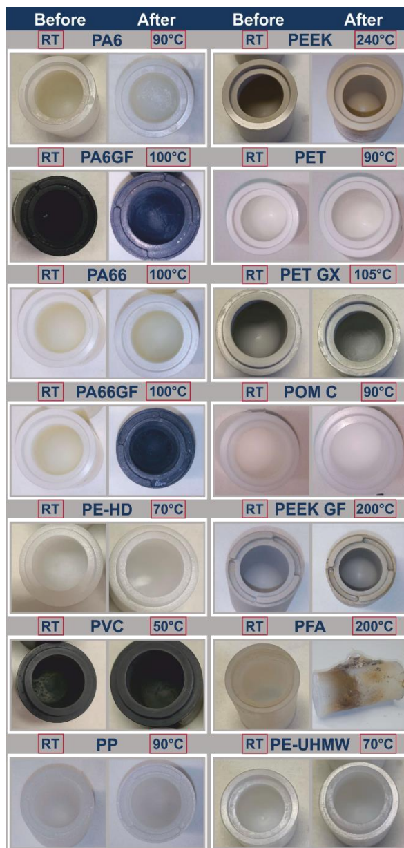
Figure S 5: Vessels before and after heating 10 °C lower than their maximum working temperature. In case of PEEK, PEEK GF and PFA, these were not heated up to his temperature, but it was limited to 240°C.
