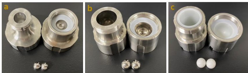
Figure S2. (a) 1.5 mL stainless-steel milling jar with two stainless-steel balls (7 mm); (b) 10 mL stainless-steel milling jar with two stainless-steel balls (10 mm); (c) 10 mL zirconium oxide milling jar with two zirconium oxide balls (10 mm).
