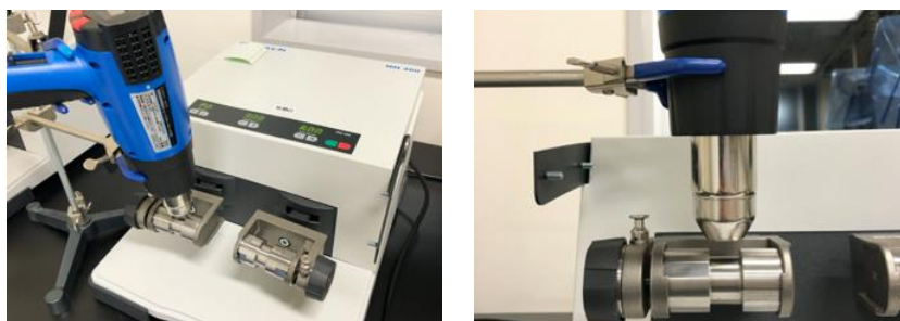
Figure S5. The set-up procedure for a heat gun on MM400.
