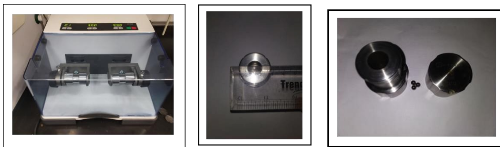
Figure S1: From left (RETSCH 400™) High Energy Mixer Mill, 27 mm stainless steel jar and 5 mm stainless steel balls.
