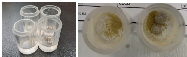
Figure S1. (left) Empty PMMA milling jar with two SS milling balls. (right) PMMA jar with reaction mixture after the milling between chalcone ( 1 ) (1 mmol) and piperidine ( 2a ) (1 equiv.) at 30 Hz milling frequency. The final reaction mixture was in a free-flowing powder form.
