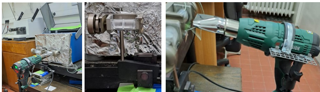
Figure S2. Experimental setup for conducting external heating during milling using a heat-gun (Parker side PHLG 2000 E4). The Raman probe was positioned underneath the PMMA milling jar, while the heating device was placed laterally. A thermocouple was put around the external milling jar surface to monitor the temperature. The temperature was followed using both a multimeter and the built-in electronic gauge on the heat gun.
