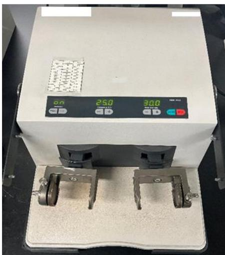
**Figure S1.** Retsch MM400 used in this study.
