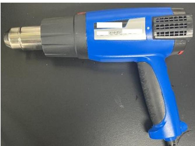
**Figure S3.** The temperature controllable heat gun Takagi HG-1450B used in this study.
