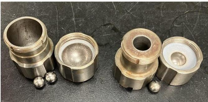
**Figure S2.** Stainless jar (25 mL and 5 mL) and balls (10 mm) used in this study.
