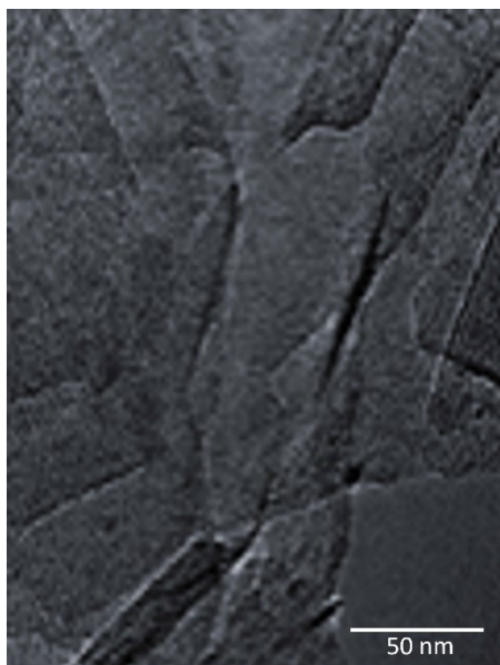
Figure 20S. a) SEM image of recovered MLG-Ru
