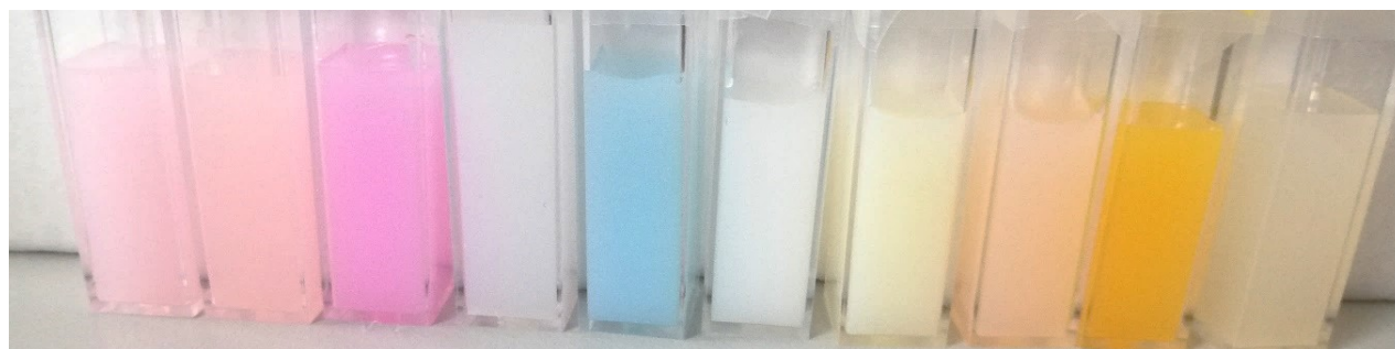
Figure S 3: Photograph of dye-MSN@TiO 2 . From left to right: R6G-MSN@TiO 2 , SG-MSN@TiO 2 , RhB-MSN@TiO 2 , C307-MSN@TiO 2 , NBA-MSN@TiO 2 , 1,3,6-naphthalene sulfonate NTS-MSN@TiO 2 (UV-Tracer, therefore no color visible and no fluorescence detected), Fluo-MSN@SiO 2 @TiO 2 , Rubpy-MSN@TiO 2 , Rubpy@SiNPs@SiO 2 , Fluo-MSN@TiO 2 .
