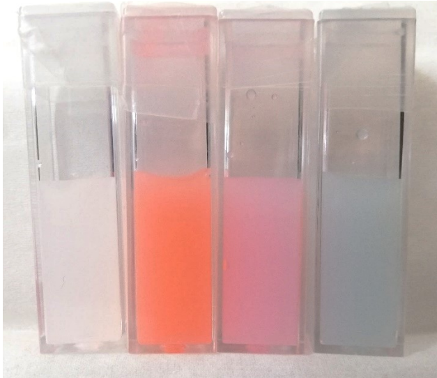
Figure S 4: Photograph of pure titania particles, SG-MSN@TiO 2 , R6G-MSN@TiO 2 , R800-MSN@TiO 2 (from left to right).
