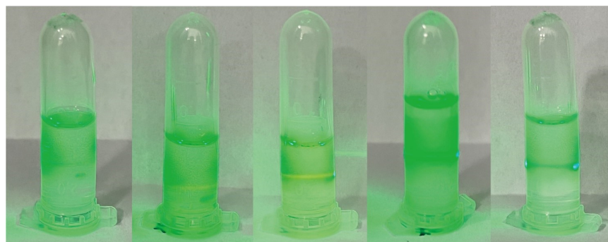
Fig. S2 The optical path under laser irradiation of T161, T151, T154, S17000 and S24000 in Isopar L.
