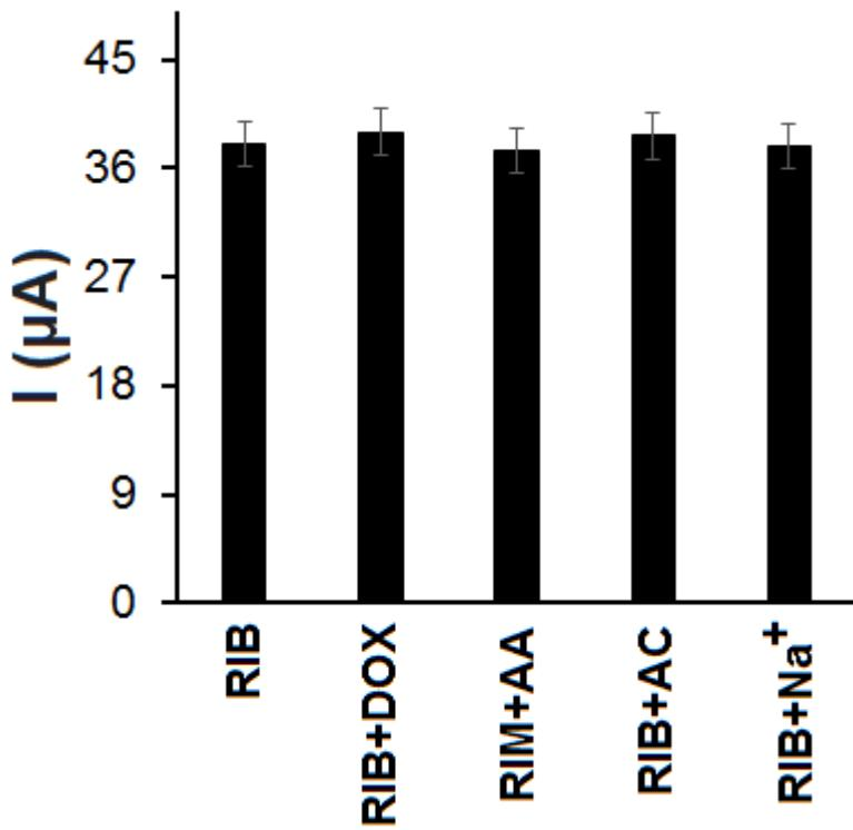
**Fig. S1.** Detected current of  $5 \mu\text{mol L}^{-1}$  RIB at  $\text{SiO}_2\text{-OMC/CPE}$  in PBS (pH 7.0) upon the addition of  $5 \mu\text{mol L}^{-1}$  doxorubicin (DOX), ascorbic acid (AA), acetaminophen (AC), and  $\text{Na}^+$ .
