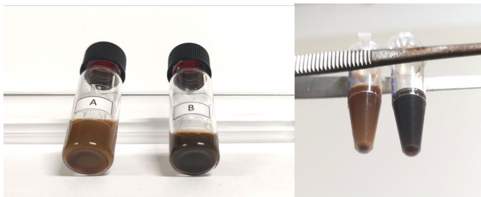
Figure S5. Dispersion stability of IONPs (4 mg/mL, sonicated for 3 min (3 times), stored for 12 hrs: Sample A MNPs@CA- \beta CD physically assembly oil bath (Table S1, entry 1); Sample B MNPs@CA- \beta CD physically assembly MW/US (Table S1, entry 2)
