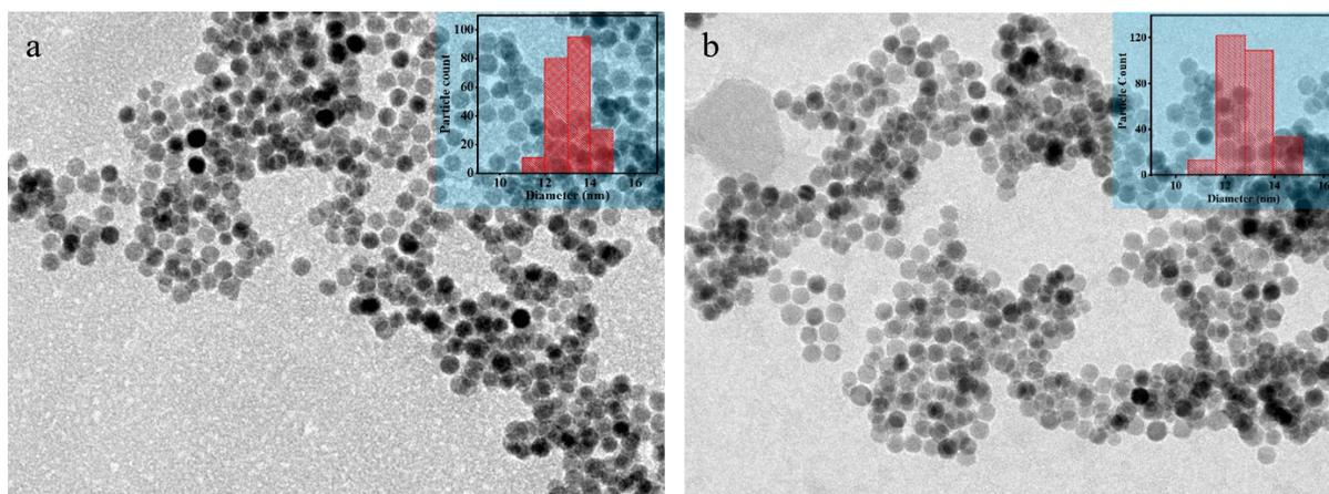
Figure R6: TEM images of the NTA@SPIONs (a) before and (b) after  $\text{Cr}_2\text{O}_7^{2-}$  adsorption.
