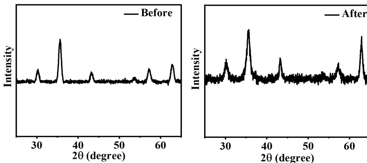
Figure R5: XRD of the NTA@SPIONs before and after Cr<sub>2</sub>O<sub>7</sub><sup>2-</sup> adsorption.
