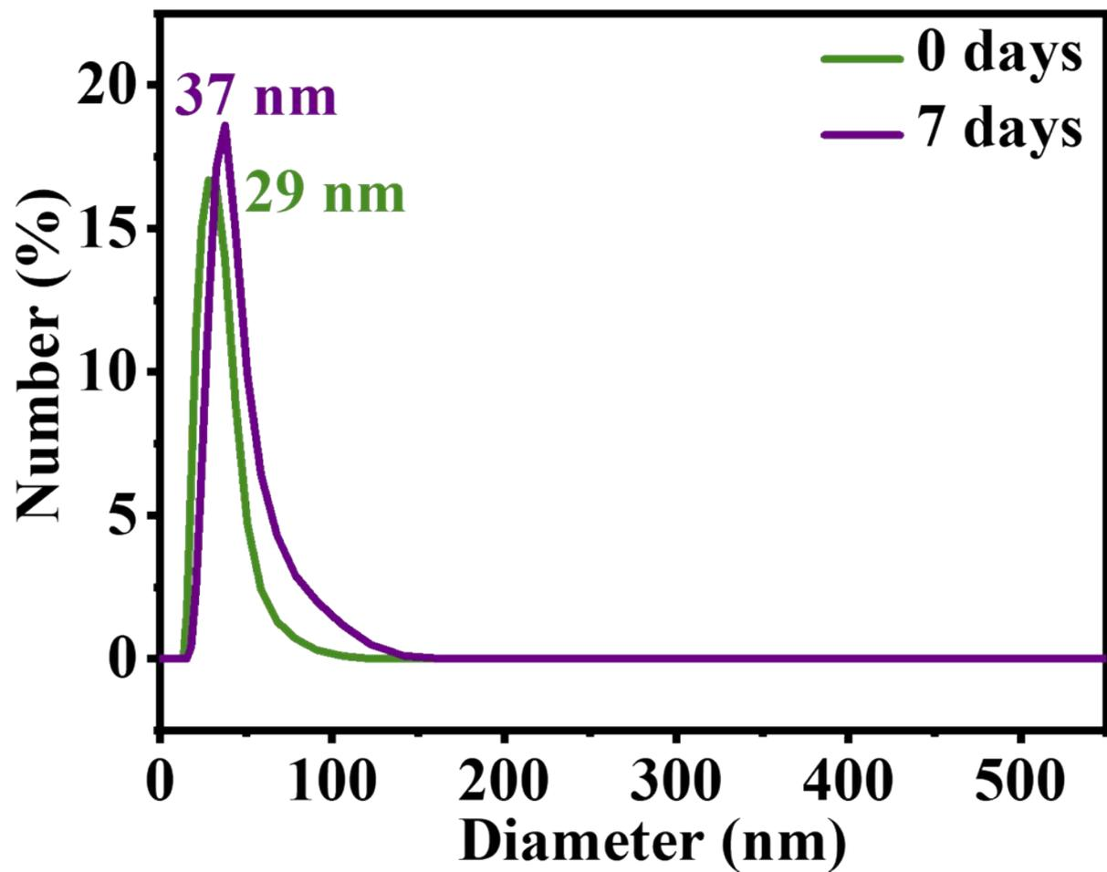
Figure S2: Hydrodynamic particle size measurement (DLS) of NTA@SPIONs immediately after preparation and after a gap of seven days.
