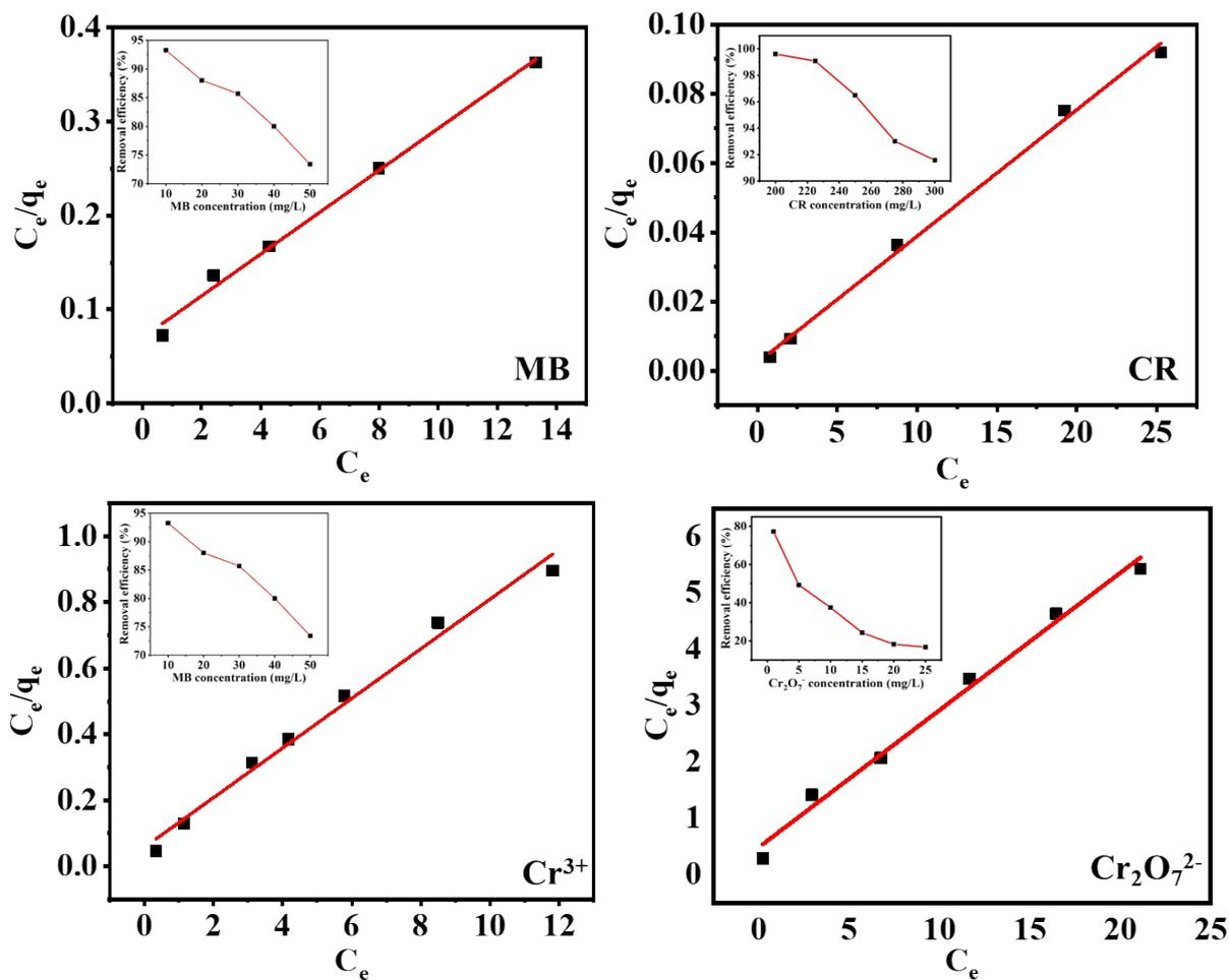
Figure S3: Langmuir isotherm fitting for MB, CR, Cr<sup>3+</sup> and Cr<sub>2</sub>O<sub>7</sub><sup>2-</sup>. Inset shows the dependency of removal efficiency on adsorbate concentration.
