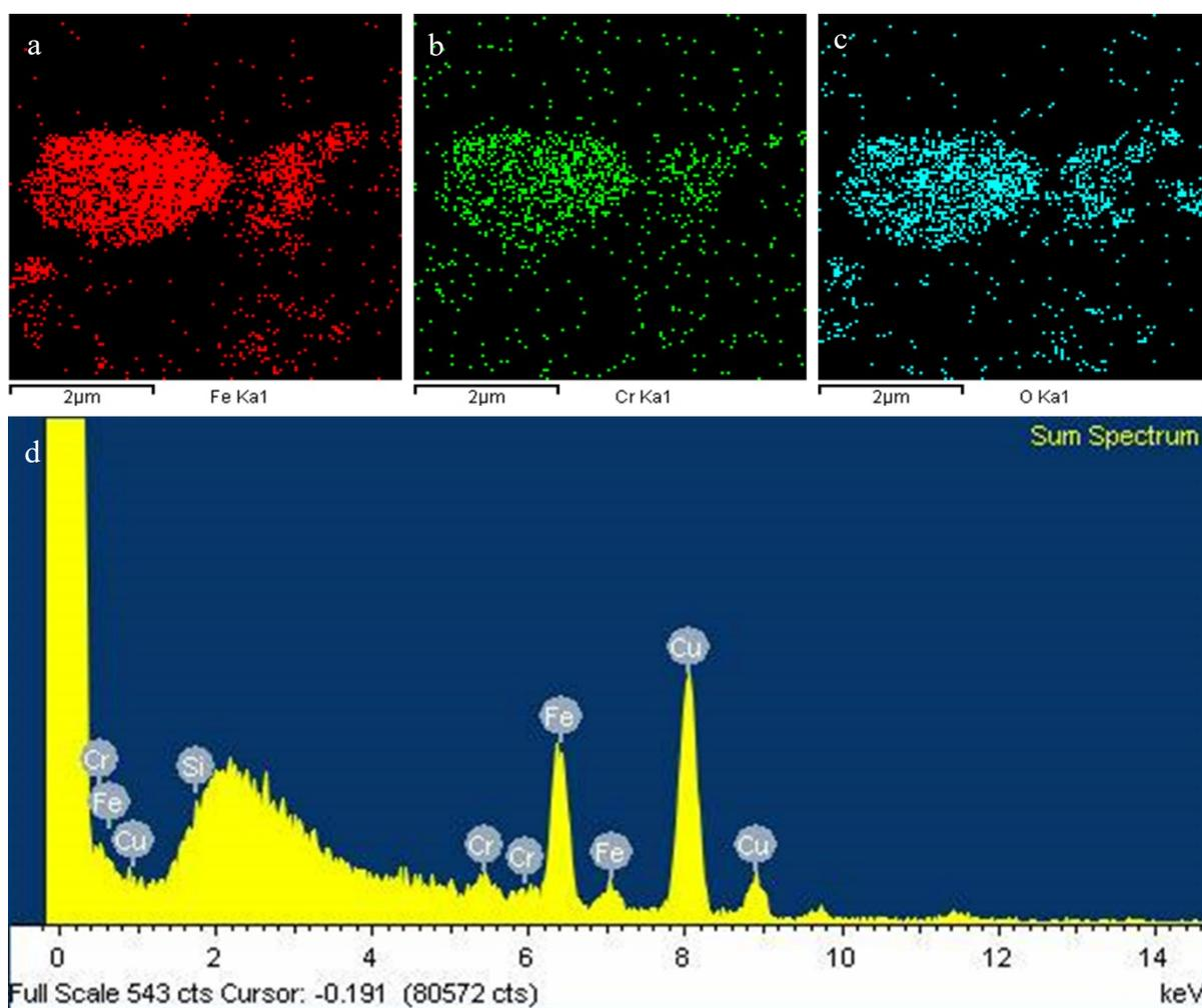
Figure R7: EDS elemental mapping of the NTA@SPIONs after  $\text{Cr}_2\text{O}_7^{2-}$  adsorption at pH 4 (a) Fe, (b) Cr, and (c) O. (d) EDS spectrum of the NTA@SPIONs after  $\text{Cr}_2\text{O}_7^{2-}$  adsorption.
