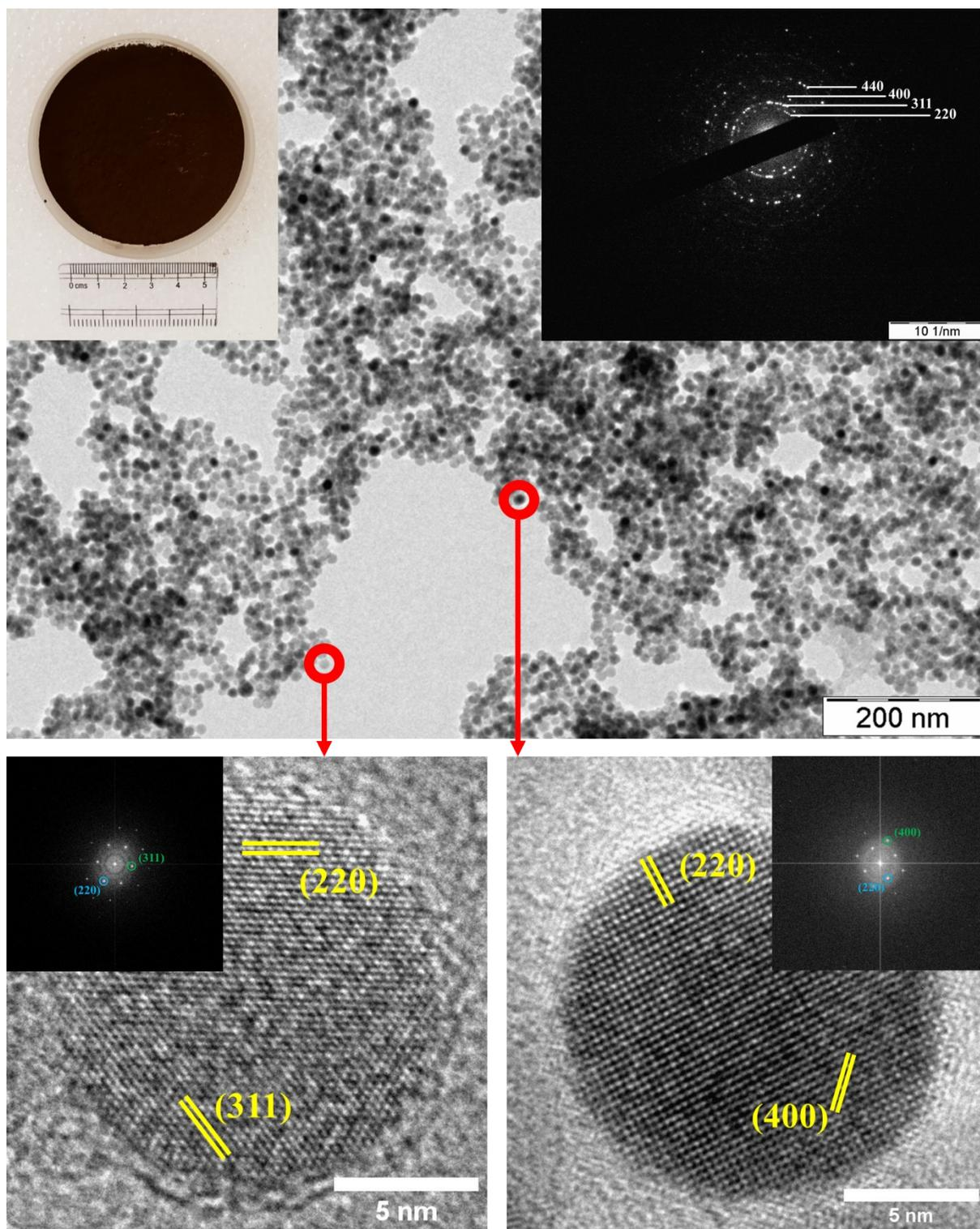
Figure S1: Large-area TEM image of NTA@SPIONs with a photograph of material obtained from a single batch (left inset) and indexed SAED pattern matching with spinel magnetite phase (right inset). HRTEM and corresponding FFT (inset) for a particle with (a) light, and (b) dark contrast. Indexed planes match with the spinel magnetite phase.
