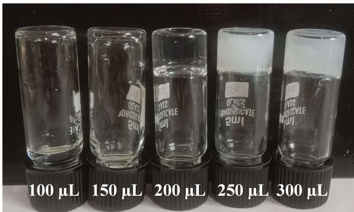
Figure S19. Digital images showing the stability of zn-inosine metallogel at different NaOH Concentrations from 100 \mu\text{L}/\text{ml} to 300 \mu\text{L}/\text{ml} .
