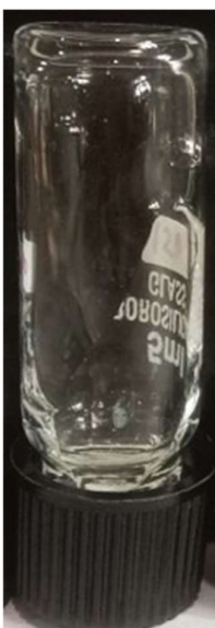
Figure S7. Digital image showing the formation of viscous sol at 20 mM concentration of both the precursors.
