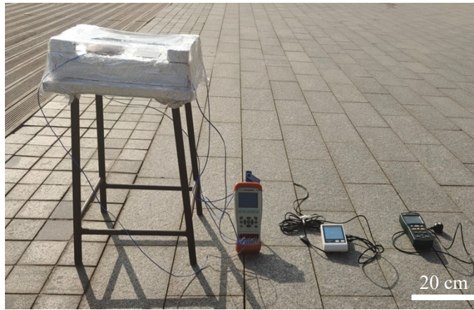
Figure S11: Cooling device physical map. From left to right, there is polystyrene foam supported by stool, multi-channel thermometer, hygrometer, and solar power meter.
