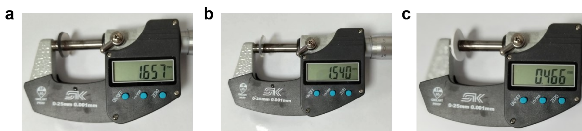
5 Fig. S3 Thickness of (a) ISGHE and (b) glass fiber separator.
