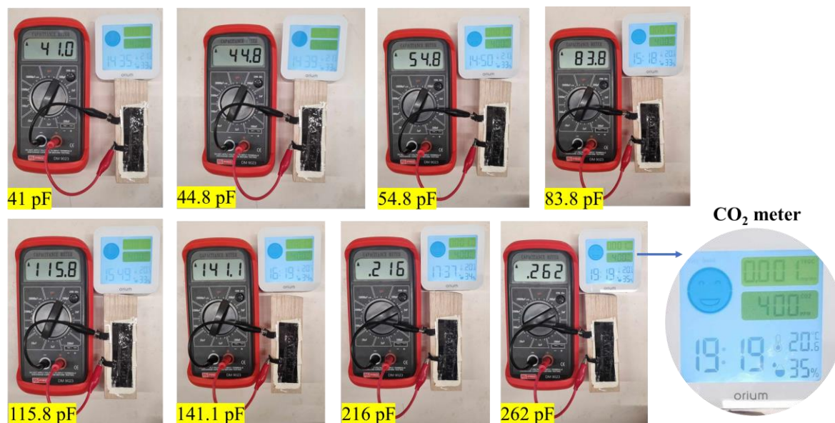
Figure S3. Temporal variation of capacitance for A-CNFs@DE exposed to 400 ppm CO 2 .
