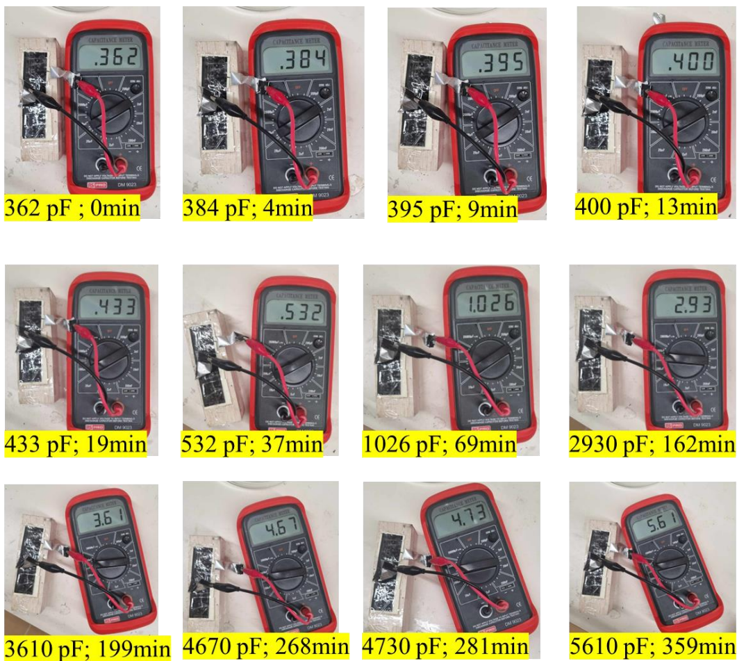
Figure S4. Temporal variation of capacitance for A-CNFs-DBU@DE exposed to 400 ppm CO 2 .
