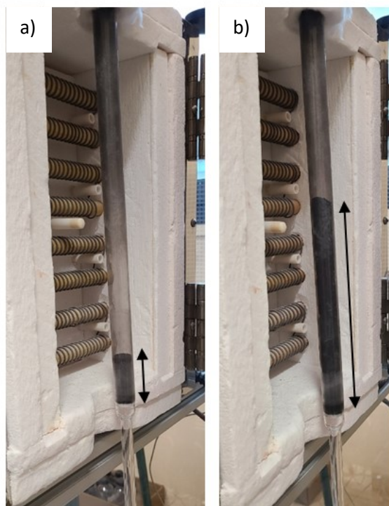
Figure S5: Quartz reactor filled with a) fresh and b) spent Fe/C catalyst. Black arrow is for catalyst bed height: 5 cm before cracking, 18 cm after biogas reforming, T=950^{\circ}\text{C} , 1 bar, \text{CH}_4:\text{CO}_2:\text{N}_2 2:1:1, 300\text{ mL min}^{-1} .
