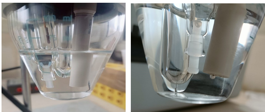
Fig. S1 Left: Photograph of three-electrode electrochemical cell for overall water splitting; Right: Enlarged view of cell showing bubbling of gases
