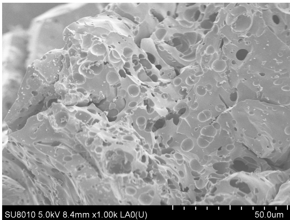
Figure S3. SEM image of annealed Ru NPs.
