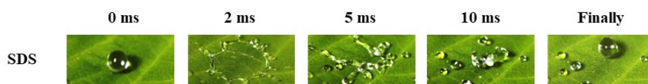
Fig. S7 The deposition of a high-speed ( \sim 1.98 \text{ m s}^{-1} ) SDS droplets on soybean hydrophobic leaf surface.
