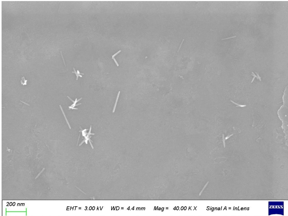
Fig. S3 The FESEM image of the Te NWs that were grown for 5 minutes.
