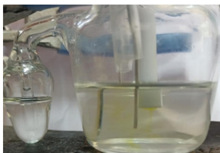
Figure SI-16. Yellow colour of the solution that appeared at 1.7 V.
