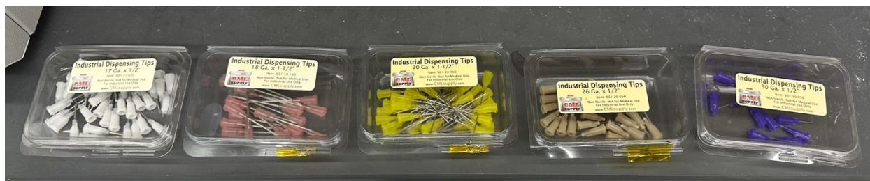
Figure S27. A depiction of most of the needle gauge sizes used in synthesis.
