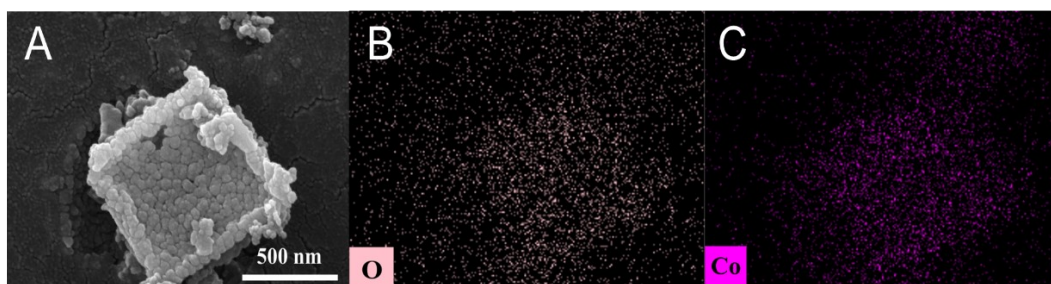
Figure S2 SEM images (A) and EDS mapping of \text{Co}_3\text{O}_4 (B),(C).
