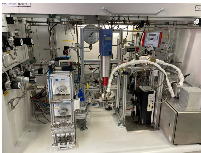
Figure SI-2: Experimental set-up with 200 ml reactor for in-situ FTIR monitoring during alkene hydroformylation.
