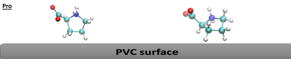
Figure S10: Configuration of the adsorbed Pro residues onto the PVC surface
