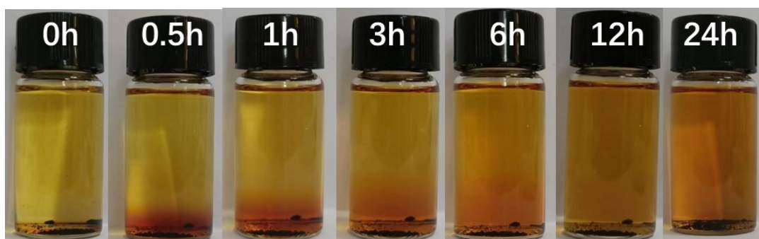
Figure S25. The iodine releasing process of I_2@JLNU-313 from ethanol solution.
