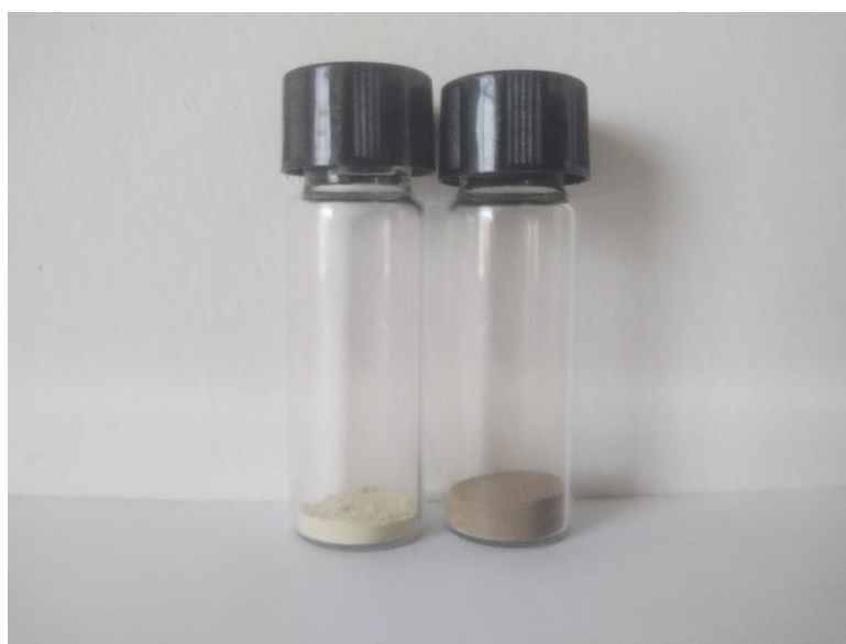
Figure S2. photographs of bulk and porous g-C 3 N 4 with same mass.
