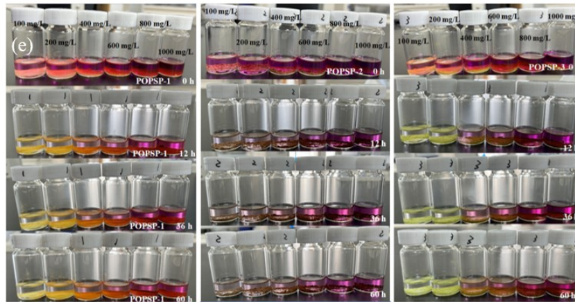
Fig. S14. (a) Iodine uptake performance of POPSP-1, POPSP-2, and POPSP-3 in n -hexane solution. The Langmuir adsorption model and Freundlich adsorption model for POPSP-1 (b), POPSP-2 (c), and POPSP-3 (d). (e) Three polymers were immersed in iodine/hexane solutions of different concentrations.
