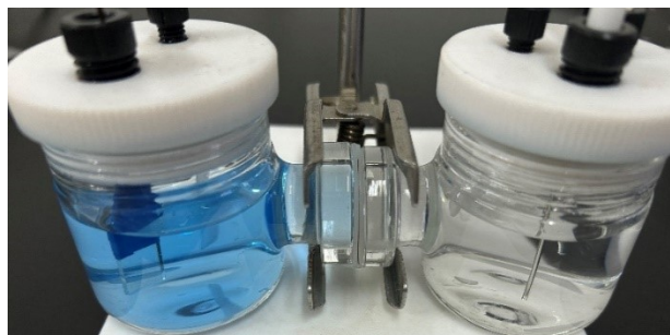
Fig. S16 Picture of the two-compartment electrochemical cell used for CPE experiments; 0.1 M PBS (pH 8.0) containing 1 mM of 1 was used as electrolyte and potential was controlled at 1.60 V vs. NHE.
