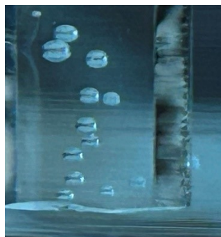
Fig. S17 The oxygen bubbles generated on the surface of ITO electrode during CPE test of 1 .
