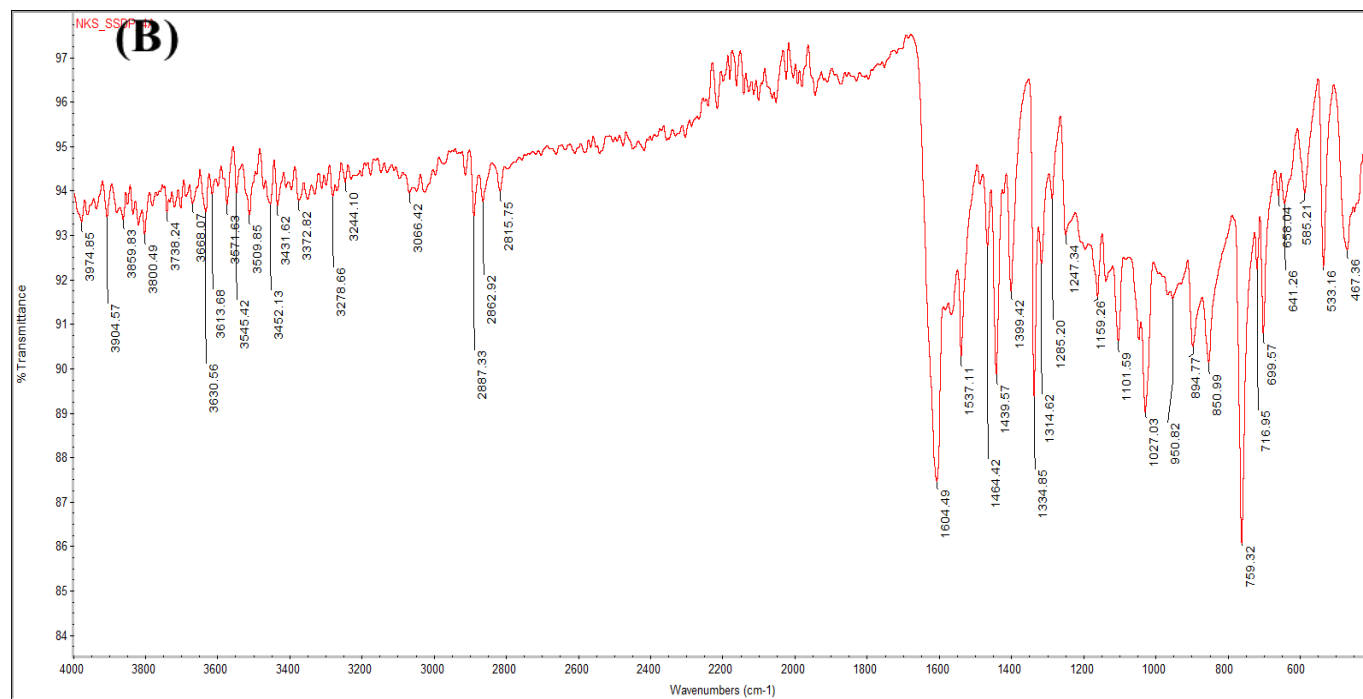
Figure S5. (A) FTIR Spectra of Ligands 4a; (B) FTIR Spectra of Cu complex 4a.
