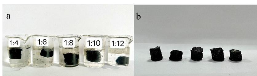
Fig. S2 The photographs of reduced graphene oxide hydrogels(a) and aerogel(b) with different mass ratio of GO to L-Cys.
