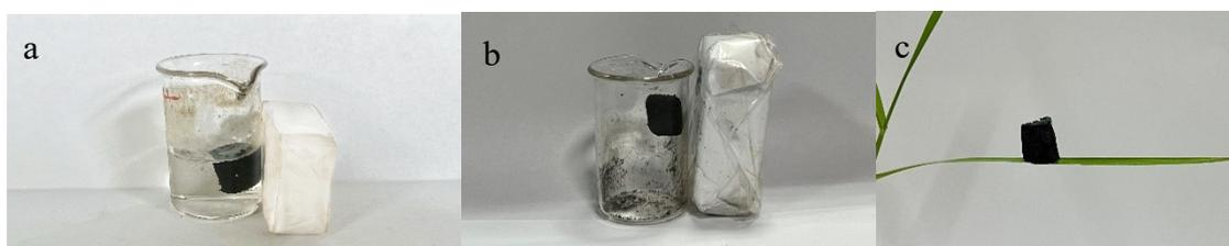
Fig. S4 The photographs of  $\text{Fe}_3\text{O}_4/\text{ZIF-8}/\text{rGO}$ (FZG15) hydrogel(a), aerogel(b) and it placed on thin leaf(c).
