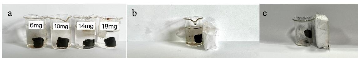
Fig. S3 The photographs of  $\text{Fe}_3\text{O}_4/\text{rGO}$  hydrogel with various dosages of  $\text{Fe}_3\text{O}_4$  (a),  $\text{Fe}_3\text{O}_4/\text{rGO}$  hydrogel(b) and  $\text{Fe}_3\text{O}_4/\text{rGO}$  aerogel(c) adding 10 mg  $\text{Fe}_3\text{O}_4$ .
