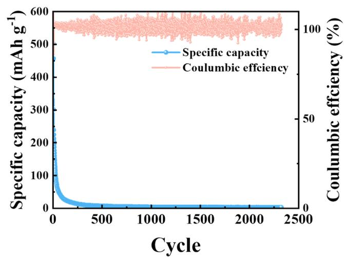
**Figure S5** Cycle performance of C@Sn<sub>x</sub>S<sub>y</sub>@HCS in 1 M NaClO<sub>4</sub> in EC:PC:DMC = 1:1:1 electrolyte.
