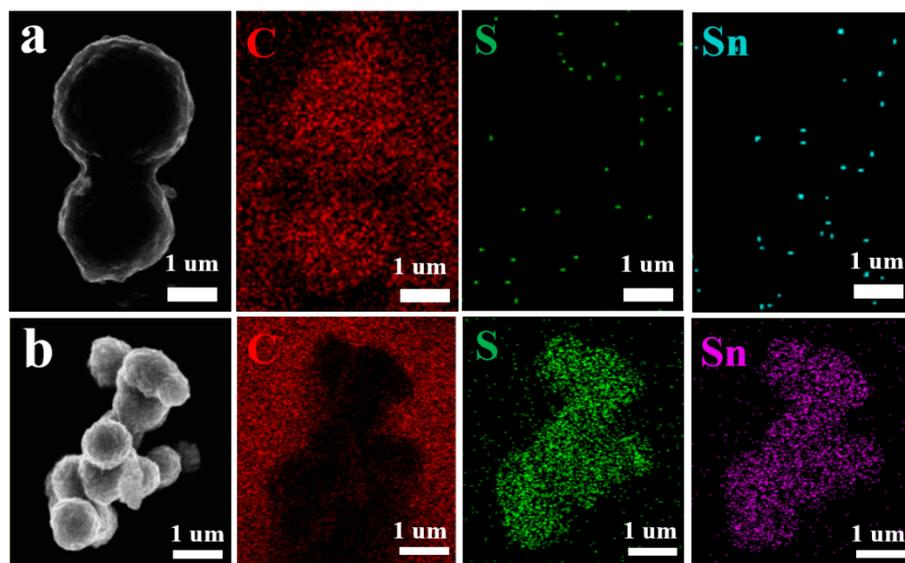
**Figure S1** EDS analysis of a) HCS and b)  $\text{Sn}_x\text{S}_y@$ HCS.
