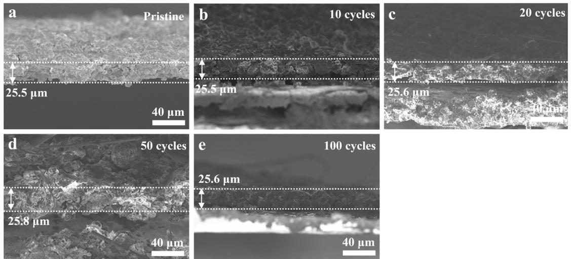
**Figure S6** The thickness evolution of the hard carbon anode.
