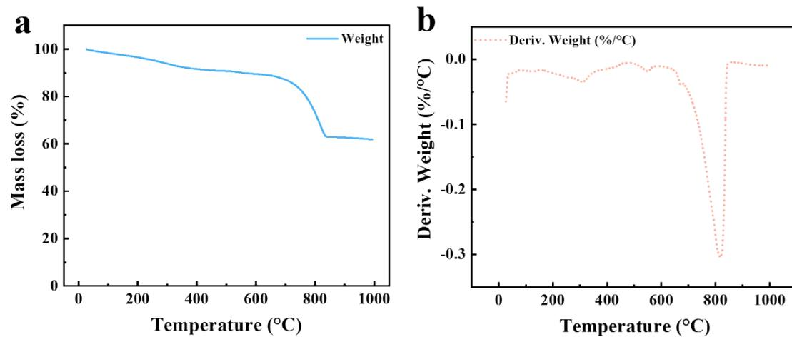
**Figure S3** a) TGA and b) DTG curves of C@Sn<sub>x</sub>S<sub>y</sub>@HCS
