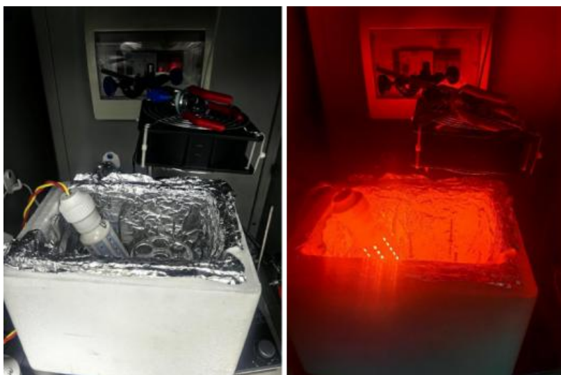
Figure S1 Reaction setup (30 W or 15 W red LEDs)
