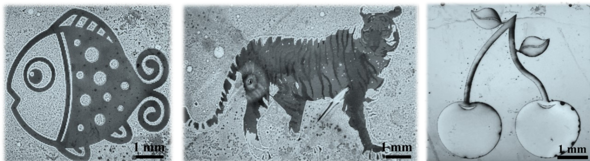
Figure S6 Optical microscope photographs of Goldfish, Tiger and Cherries on glass substrates based on the patterning process.
