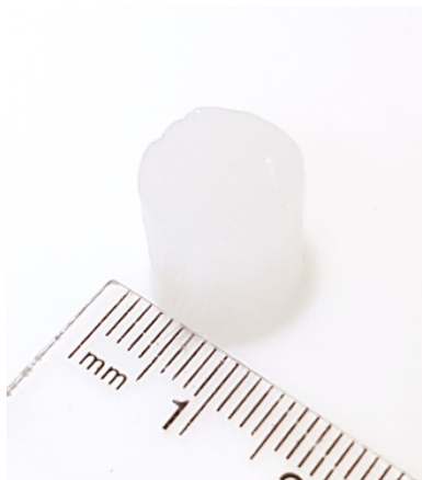
Figure S1. Macroscopic aspect of a pristine calcium alginate hydrogel cylinder before NPs synthesis.
