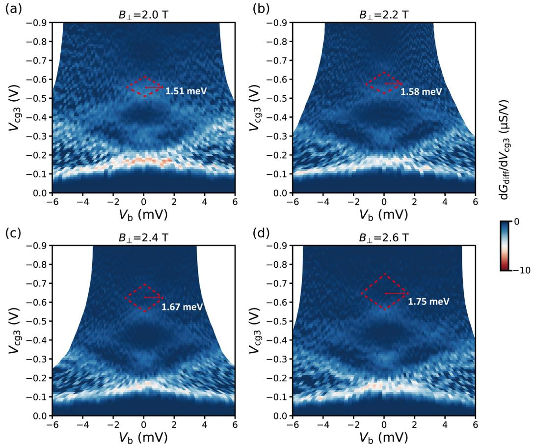
FIG. S7. Bias-spectroscopy measurements of QPC3 at different  $B_{\perp}$ . Red dashed lines denote the diamond formed by the second subband with finite Zeeman energies. The extracted Zeeman energies of the second subband at different  $B_{\perp}$  are displayed in Figure 3(g) of the main article.
