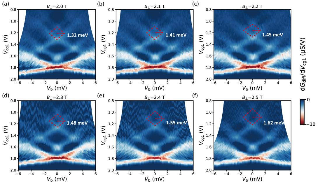
FIG. S5. Bias-spectroscopy measurements of QPC1 at different perpendicular magnetic fields  $B_{\perp}$ . Red dashed lines denote the diamond formed by the second subband with finite Zeeman energies. The extracted Zeeman energies of the second subband at different  $B_{\perp}$  are displayed in Figure 3(e) of the main article.
