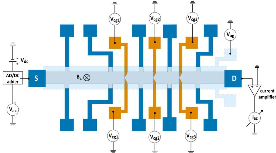
FIG. S2. Measurement setup for QPC measurements. An ac voltage  $V_{ac}$  and a dc voltage  $V_{dc}$  are summed up with a summing module before feeding into the source lead, while the ac current  $I_{ac}$  is measured with the help of a current pre-amplifier. Three QPCs are defined with three pairs of constriction gates with voltage  $V_{cg1}$ ,  $V_{cg2}$  and  $V_{cg3}$ . The accumulation gate with voltage  $V_{ag}$  is used to tune the carrier density in the device globally.
