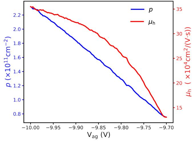
FIG. S3. Carrier density  $p$  and hole mobility  $\mu_h$  in the Ge quantum well as a function of the accumulation gate  $V_{ag}$ . Corresponding data are measured from the Hall bar structure with a measurement setup shown in Figure S1. The accumulation gate is fixed at  $V_{ag} = -10$  V in all the QPC measurements.
