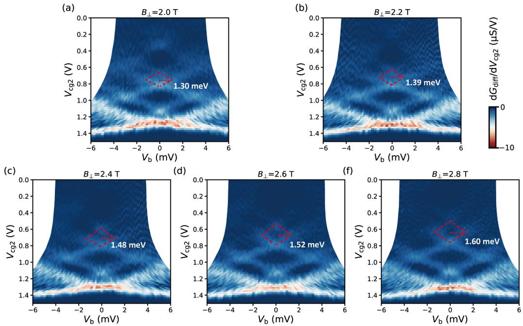
FIG. S6. Bias-spectroscopy measurements of QPC2 at different  $B_{\perp}$ . Red dashed lines denote the diamond formed by the second subband with finite Zeeman energies. The extracted Zeeman energies of the second subband at different  $B_{\perp}$  are displayed in Figure 3(f) of the main article.
