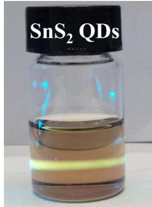
Figure S1. The photograph of the SnS 2 QD solution under an incident light beam.
