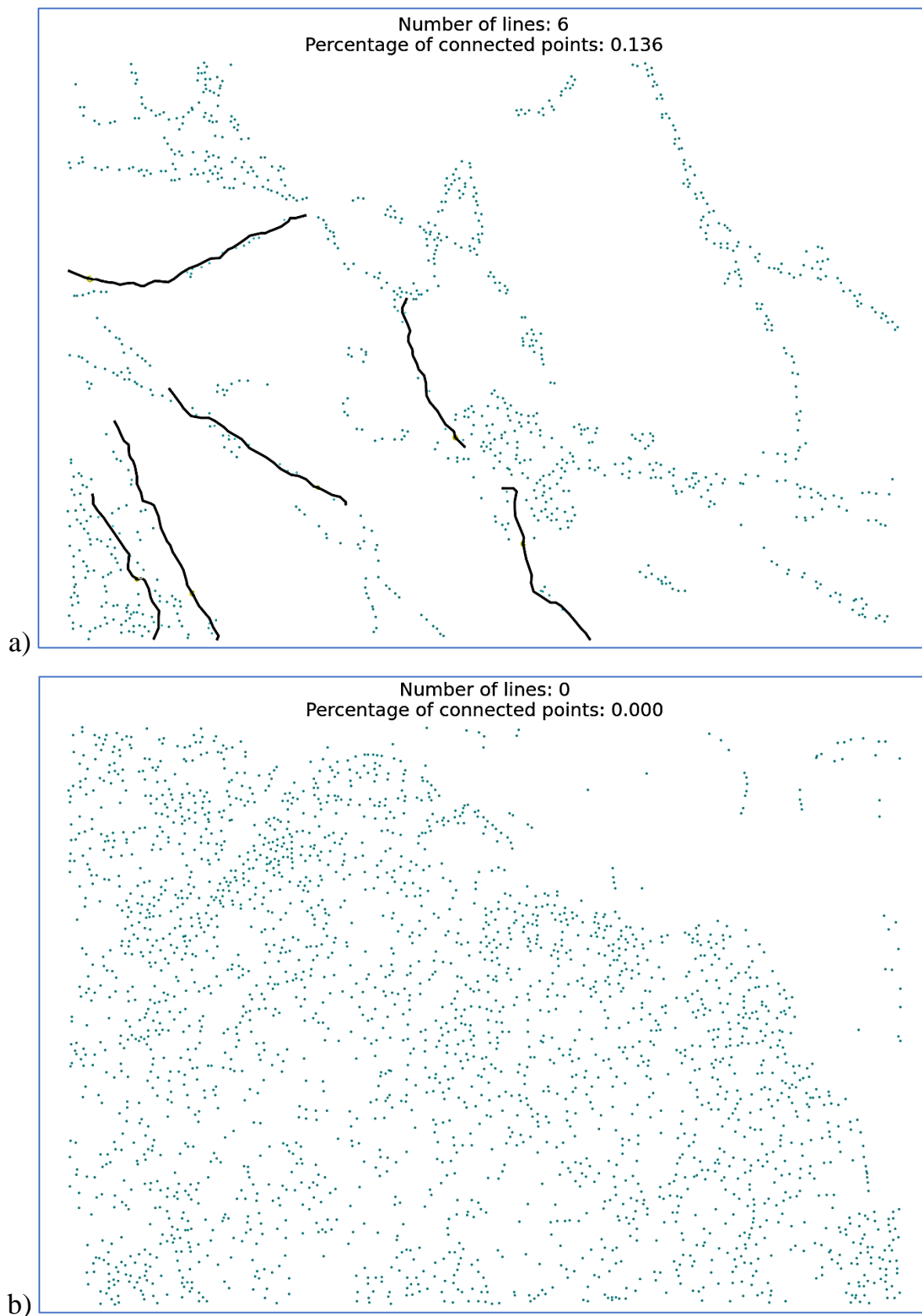
Figure 40 – Results of constructing lines for the minimum line length in the nanoparticles L_{min} = 20 . The arrangement of the particles in the SEM image: a) ordered (S1-42); b) disordered (S3-157)
