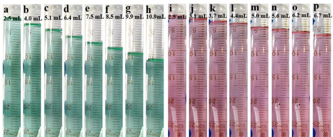
Fig. S24. Electrolyzer for polarized \text{CuCo}_2\text{O}_4 nanorods/NF(+/-) at time points 0 s, 100 s, 200 s, 300 s, 400 s, 500 s, 600 s, 700 s: (a, b, c, d, e, f, g, h) volume diagram for \text{H}_2 production; (i, j, k, l, m, n, o, p) volume diagram for \text{O}_2 production.
