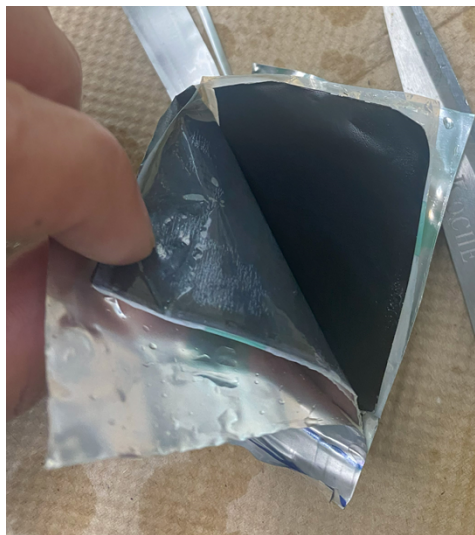
Figure S5. Visual inspection of cathode electrode after 250 cycles
